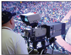
Figure 4.40 Handheld camera with large lens viewfinder and triax adapter (box hung on the back of the camera) added to "buildup" the camera into a "hard" or "studio" camera.
